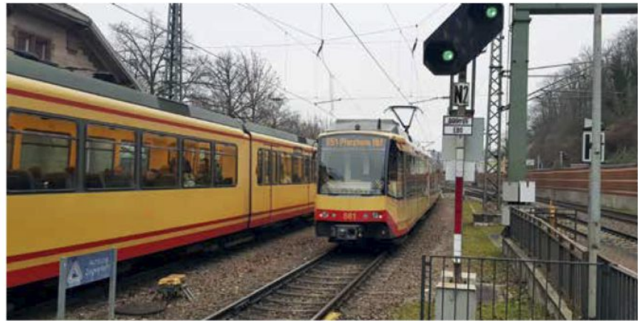
Where a tram officially becomes a train from the regulatory perspective, there is also a change of operational systems including monitoring and control.
