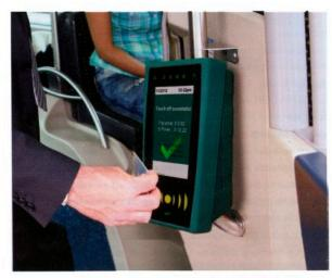
management (like MOBILEvario) and then released to the field devices via an Online Validation Server (OVS). This OVS serves real-time requests from the field devices and provides validation results as well as list updates (white/black lists).
