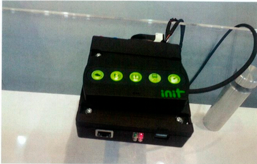
LIGHTS IN the Mobile-Eco2 alert bus operators when they're operating in a rough or irregular way.
